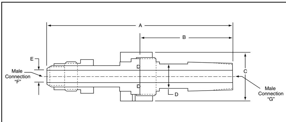
Note 1: EZ-Unions are constructed from 316 SS and are supplied with a Viton o-ring as standard.
