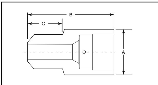
Gland and collar supplied with high pressure connections.
